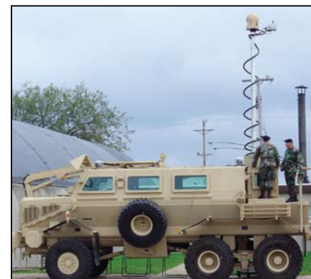
TOPMOST: The Gyrocam System, extended on its mast on RG-31 armor protected vehicles, is supporting a wide range of military missions in Iraq. LEFT: The camera system in a non-deployed position on an RG-31. TOP: The armored Buffalo vehicle also utilizes the system, as it removes explosive and other potential threats during route clearance missions. (All photographs courtesy of Gyrocam Systems, LLC)
