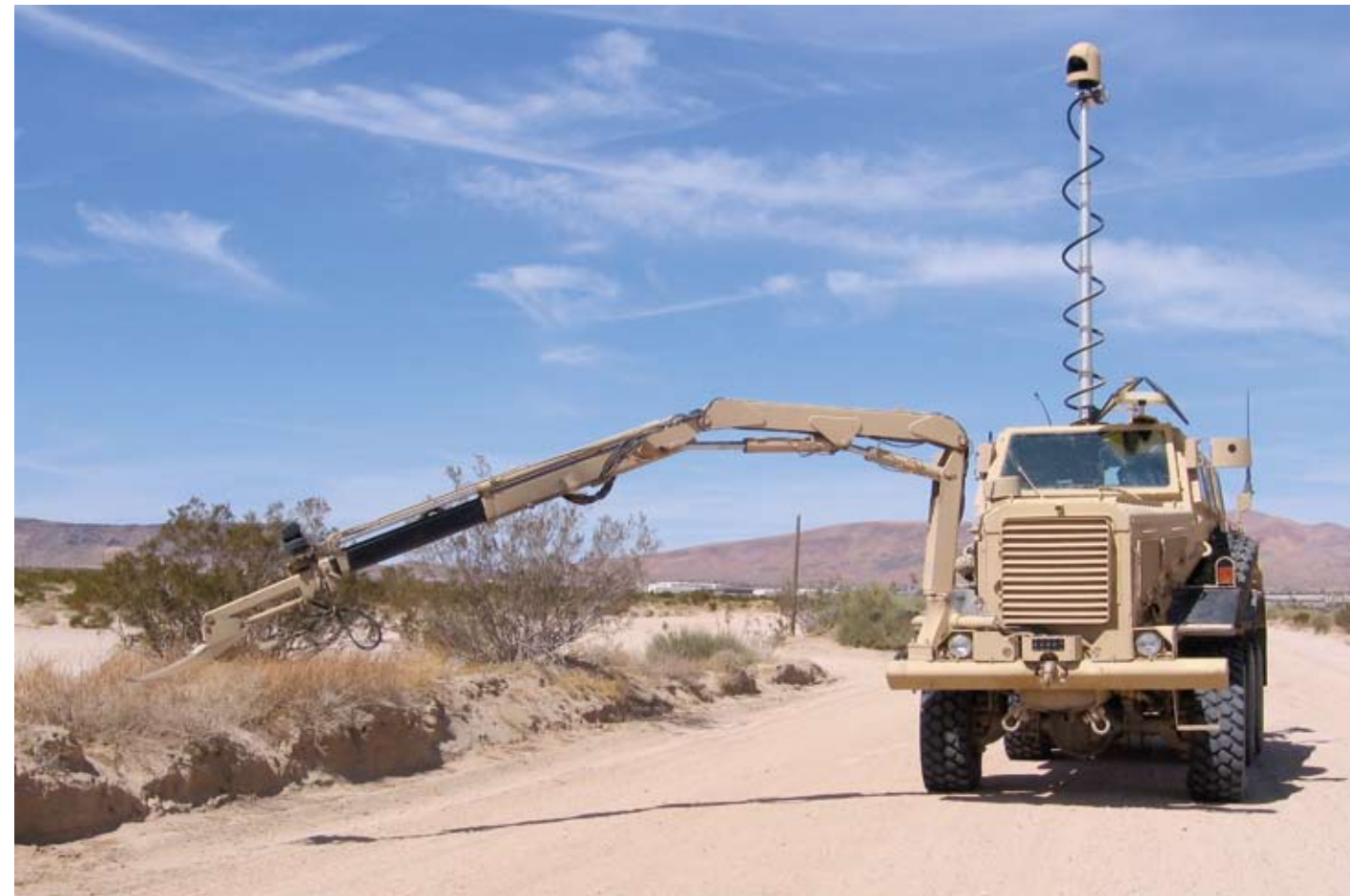
LEFT: Soldiers involved in the initial evaluation of the Hunter-Killer Project teams using the Gyrocam System. BOTTOM: The camera system fully extended, while the vehicle’s mechanical arm probes alongside the roadway. (All photographs courtesy of Gyrocam Systems, LLC)
